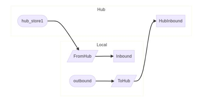
The shovels are maintained at the local virtual host, as network communications and firewalls typically allow connections from the local network to the cloud – but not the reverse. Even though network communication is one direction, a shovel can be configured to send data in either direction.
