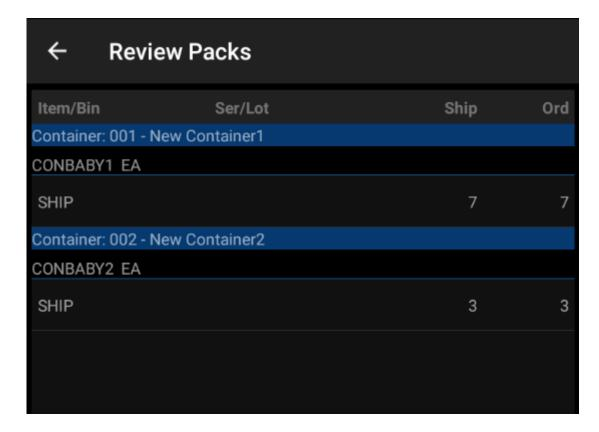
Selecting SAVE will create the containers in Acumatica. Note that Acumatica Packages are not created. Once saved, the weight can be entered, and a container label printed from the handheld. Containers can be unpacked and repacked as needed before Acumatica Packages are created. COMMIT will create the Packages on the Acumatica Shipment and change the Pick Status to Packed.
