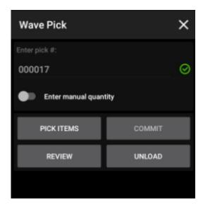
Scan or enter the wave pick number and the operator will be routed through the warehouse in an optimum manner to pick all the items included on the wave. The handheld will reflect the location, items, and combined quantities. The paper pick list will reflect the distribution of those contents among the selected shipments.
