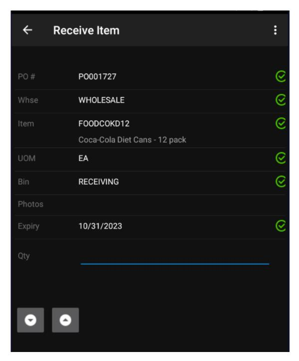
At any time in the process the operator can select REVIEW to see the items and quantities ordered and what has been received. Once the PO is fully received, each line will be marked accordingly on the
